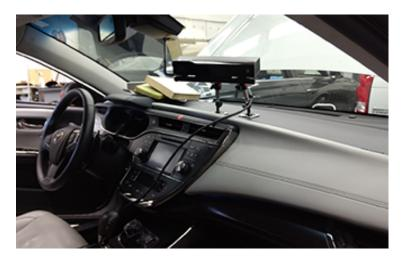
Figure 6. Placement of Kinect sensor in vehicle.
