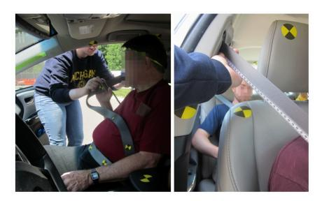
Figure 16. Locking the retractor by pulling the belt all the way out switching it from ELR to ALR.
