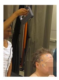
Figure 7. Scanning a participant's head with the hand-held scanner.
