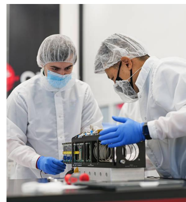
Figure 2: MiTEE-1 spacecraft developed by the University of Michigan. MiTEE-1 is a 3U CubeSat and weighs less than 4kg which greatly reduces launch and development costs.
