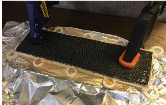
Figure 1. Molding the adhesive with glass clamped on top.
