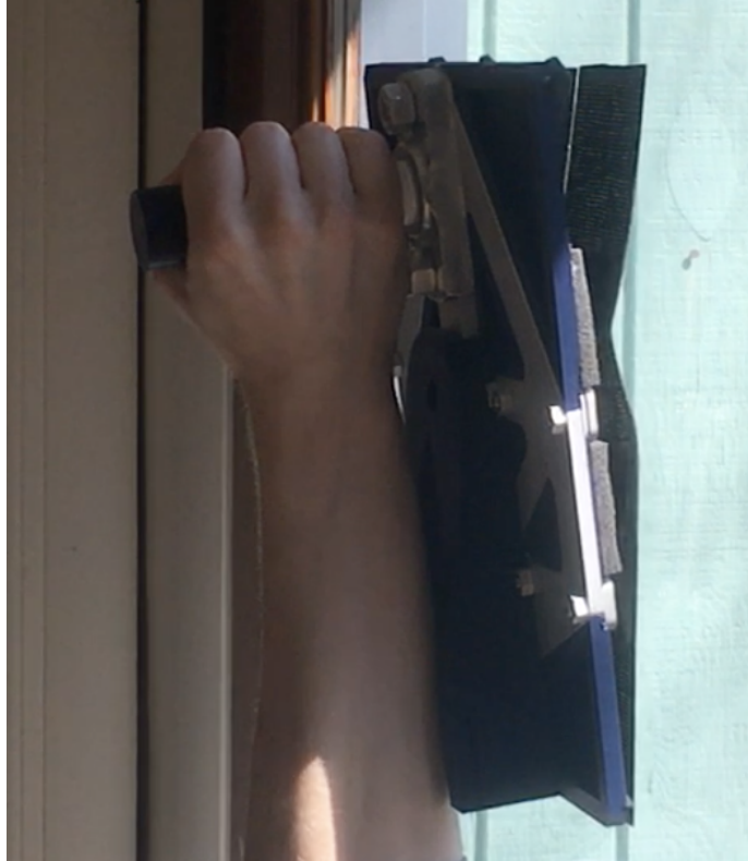
Figure 23. The tipping of the adhesive pad away from the adherend surface due to an applied moment.
