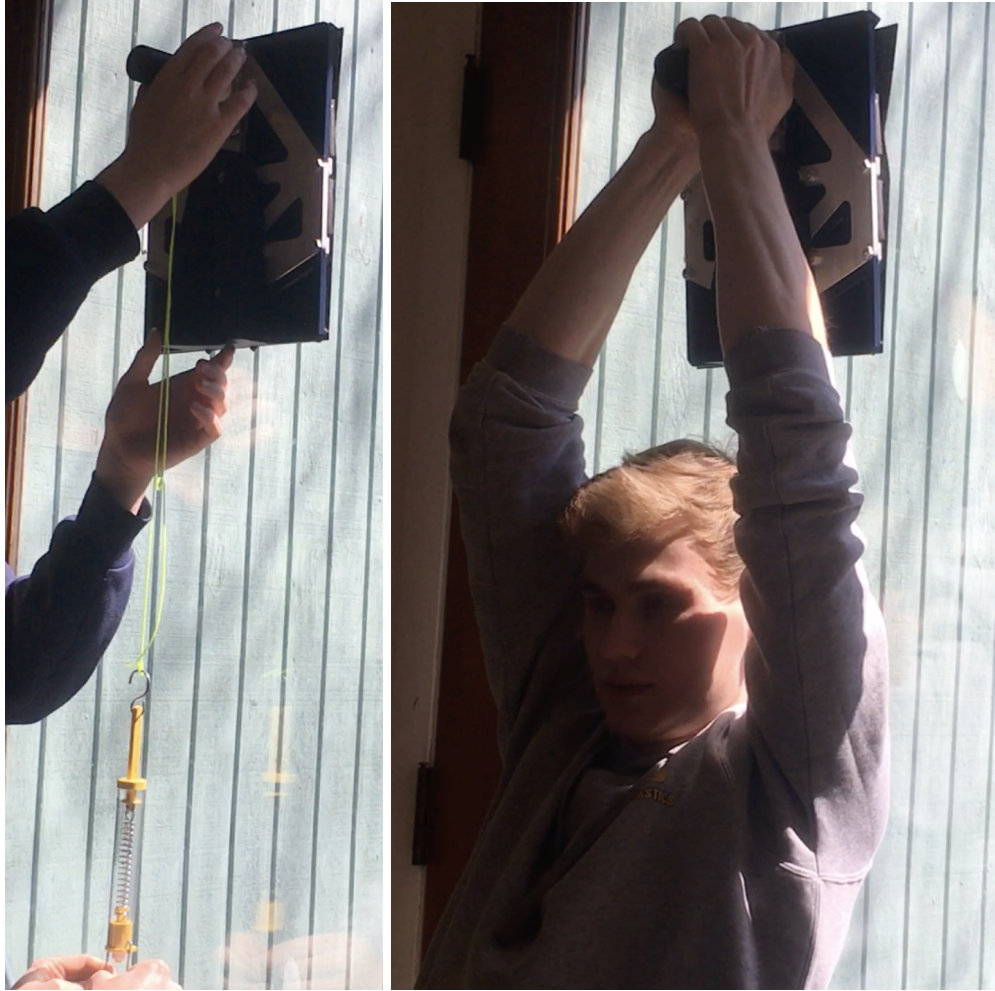
Figure 22. Testing the adhesive pad with both 50N (left) and human weight (right) loads.
