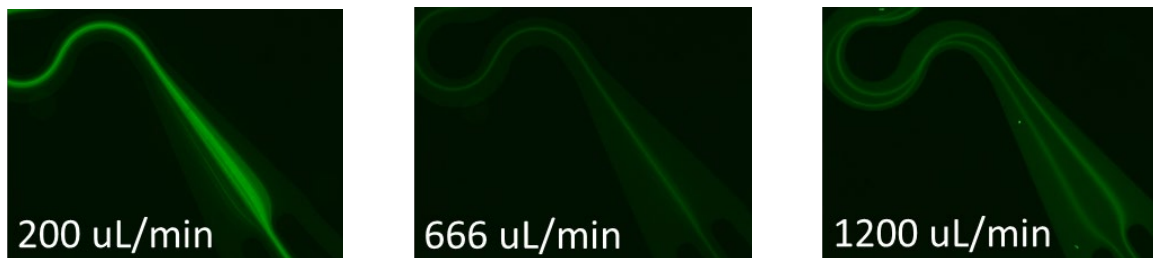
Figure 5c. Images of pre-fluoresced cells in 7 g/dL BSA in the bottom channel of the device at specified flow rates.
