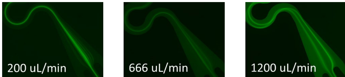
Figure 5a. Images of pre-fluoresced cells in PBS (No BSA) in the bottom channel of the device at specified flow rates.
