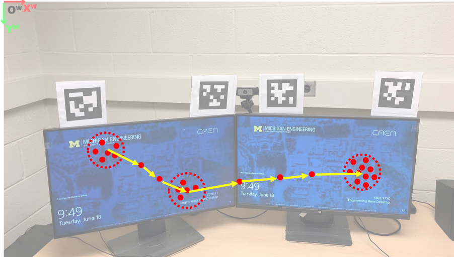
Figure 4.3: Illustration of fixations and saccades mapped on the world image. Red dots are gaze points. Red dashed circles are fixations. Yellow arrows are saccades.
