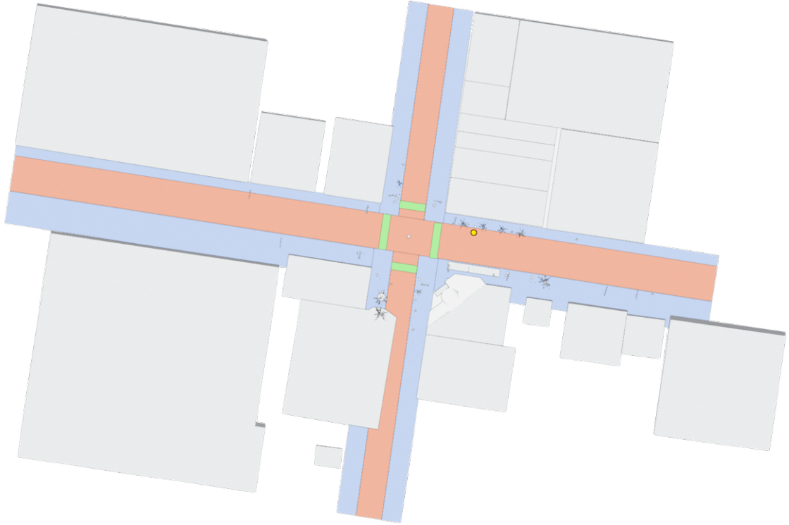
Figure 4.4: An example rendered view of a scene from the camera placed 500m away from the ground and heading towards +z direction of the global coordinate frame. Lanes, sidewalks, and crosswalks are shown in orange, blue, and green.
