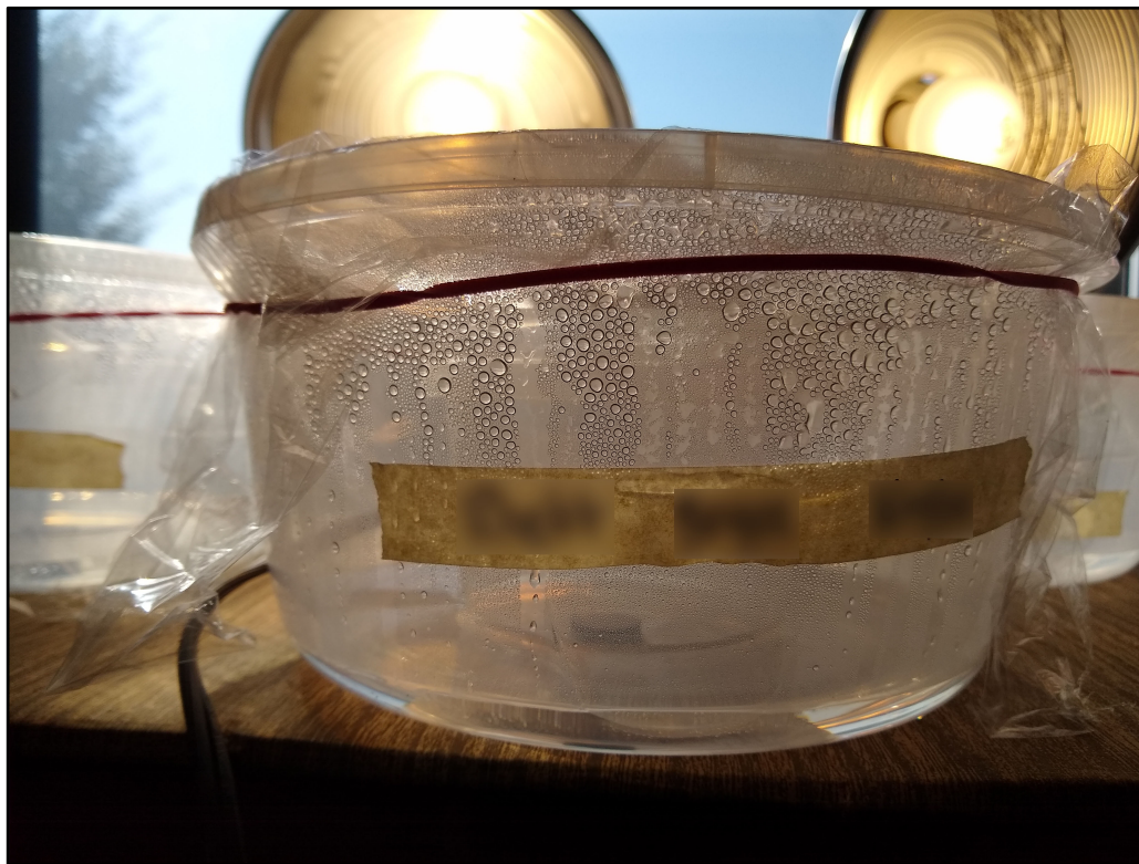
Figure 2.4: Solar stills with heat lamps in place (top); close-up of solar still with condensation (bottom) – photos from 10/15/19 (8 elapsed days, second day under the heat lamps)
