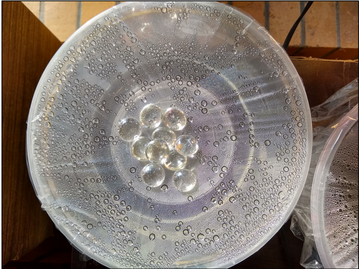
Figure 2.3: Condensation collecting on the underside of the plastic wrap covering the solar still – photo from 10/15/19 (8 elapsed days, second day under the heat lamps)
