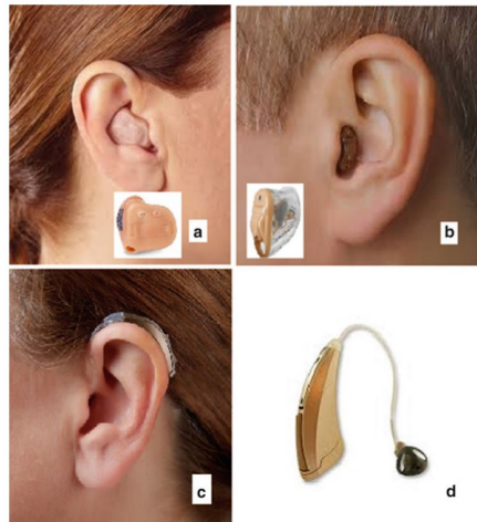
Figure 1.3: Images of different hearing aid styles. (a) and (b) demonstrate in-the-ear and in-the-canal type HAs. Behind-the-ear systems are shown in (c) and (d). This image is reused by permission from: Hearing Aids , Springer Handbook of Auditory Research, Springer International Publishing Switzerland 2016 [4].
