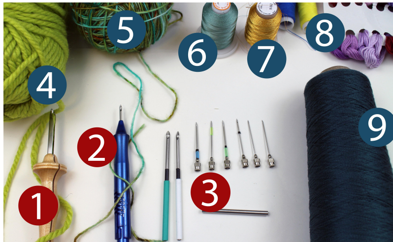
Figure 4.3: Commercially available manual punch needle tools and commonly used threads: 1-2) Oxford Punch Needle ® and Ultra Punch ® Needle, 3) a variety of punch needle heads and their interchangeable handles, 4-9) examples of threads with diverse thicknesses and material.
