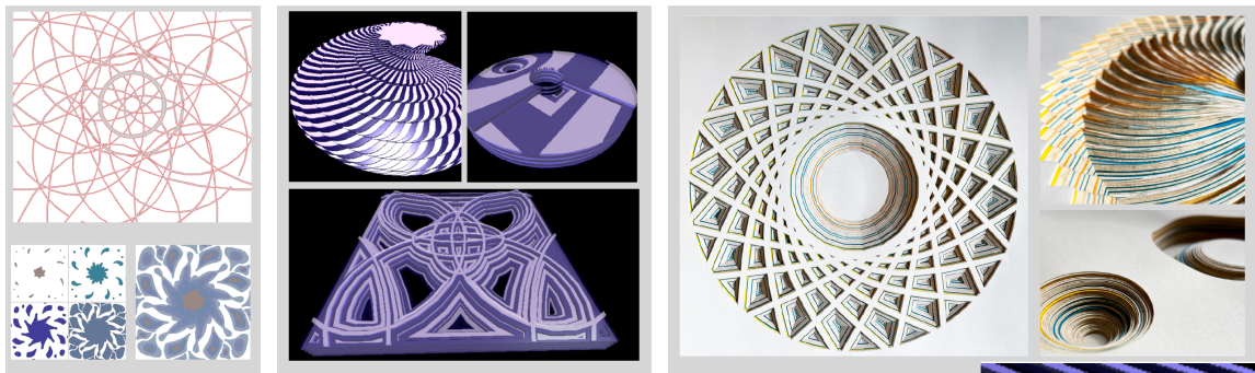
Figure 2.1: InfiniteLayer is a Python-based toolkit that assists multilayer sculpture design. It provides foundational structures and essential methods for designers to draft, import, and manipulate 2D designs (LEFT). It aids rapid prototyping by delivering 3D simulations without requiring modeling expertise. Also, it offers flexible controls over rendering settings/formats to produce designs that are compatible with a variety of fabricators (RIGHT: artwork fabricated with a laser cutter).
