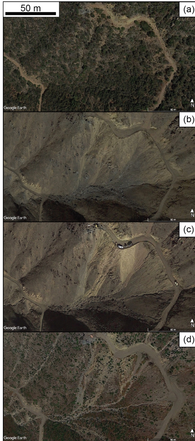
Appendix Figure E.8: Time series of Google Earth satellite images showing geomorphic change following the Woolsey Fire. a) Pre-fire image from August 12, 2018. b) Post-fire but pre-rain image from November 19, 2018. Note ravel cones on roadbed in upper-right corner of image c) Image from January 3, 2019, after the first storm. Rilling and gullying are evident. Note road maintenance equipment in the image. d) Image on August 19, 2019, following all three storms and preceding the post-fire airborne LiDAR survey by 37 days. Note vegetation regrowth. Image center 34.0593° N 118.8122° W.
