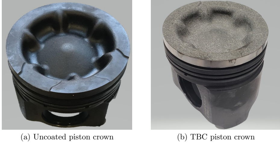
Figure 1.2: Side-by-side view of an uncoated and TBC wave piston crown.
