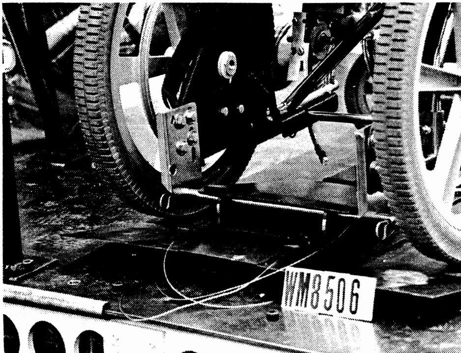
Figure 4. Close-up of modified rear tie-down mechanism.
