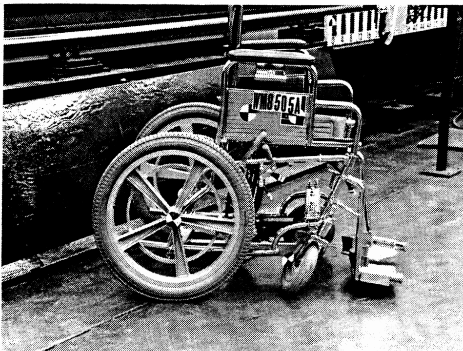
Figure 10. Collapsed wheelchair frame after impact.
