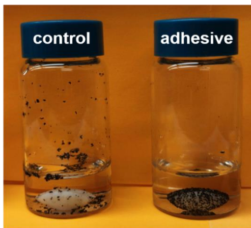
Figure 4-2. Preliminary experiments demonstrating MPs removal from water using an adhesive-coated stir bar to capture micronized rubber (~100 \mu\text{m} ) suspended in water
