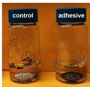
Figure A3-6. Comparing capturing MPs micronized rubber using adhesive bare (left) versus coated (right) stir bar.
