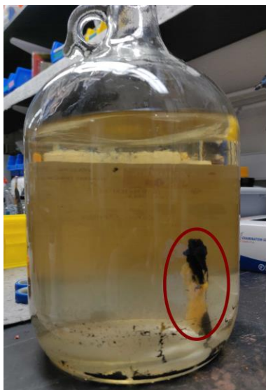
Figure 1-2. Image showing micronized rubber particles adhered onto a blob of pressure-sensitive adhesives in a solvent waste container.
