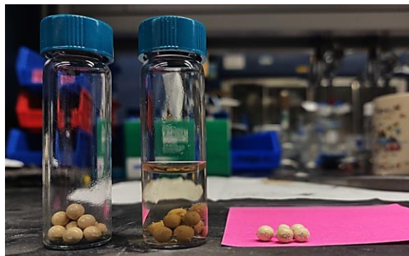
Figure A3-7. Visualization of adhesive-coated post-use 2 mm molecular sieves before (left), and after (right) MPs removal.
