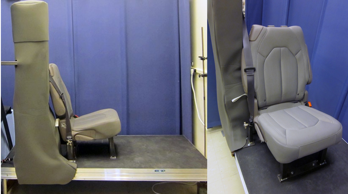
Figure 7. Mockup of minivan/ SUV second row with Chrysler Pacifica seat and C-Pillar.
