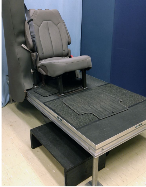
Figure 25. Changes to the seating buck to make stepping on to the buck more intuitive include adding a longer step and carpeting and floor mats
