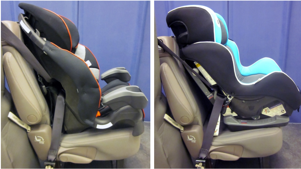
Figure 8. Forward-facing CRS Evenflo Maestro combination CRS (left) and Babytrend CV88a PROtect Series Convertible CRS (right) in side view as installed in the vehicle mockup by a study participant
