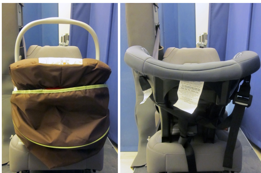
Figure 11. Rear-facing CRS Cosco APT 50 Convertible CRS (left) and Graco SnugRide 30 Infant CRS (right) in front view as installed in the vehicle mockup by a study participant
