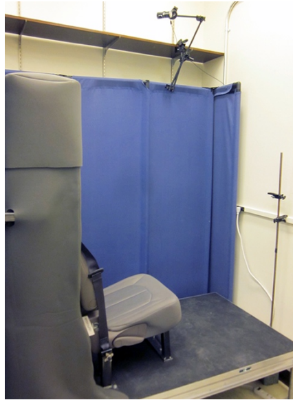
Figure 20. Mockup with video webcam mounted above and camera mount in front to document participant installations
