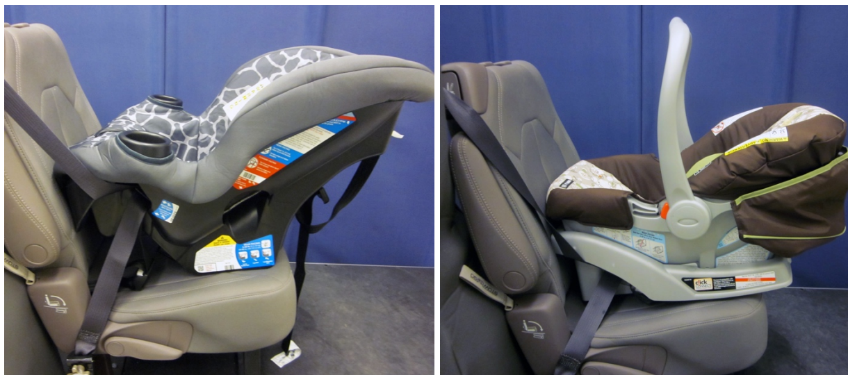
Figure 10. Rear-facing CRS Cosco APT 50 Convertible CRS (left) and Graco SnugRide 30 Infant CRS (right) in side view as installed in the vehicle mockup by a study participant
