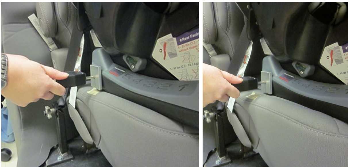
Figure 21. Investigator loading the CRS installed by the participant at the belt path with 178 N force.
