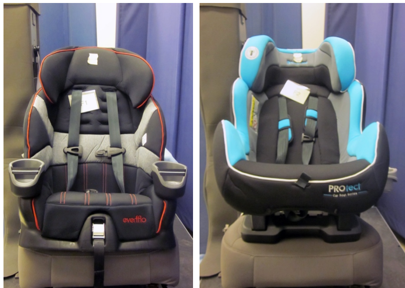
Figure 9. Forward-facing CRS Evenflo Maestro combination CRS (left) and Babytrend CV88a PROtect Series Convertible CRS (right) in front view as installed in the vehicle mockup by a study participant
