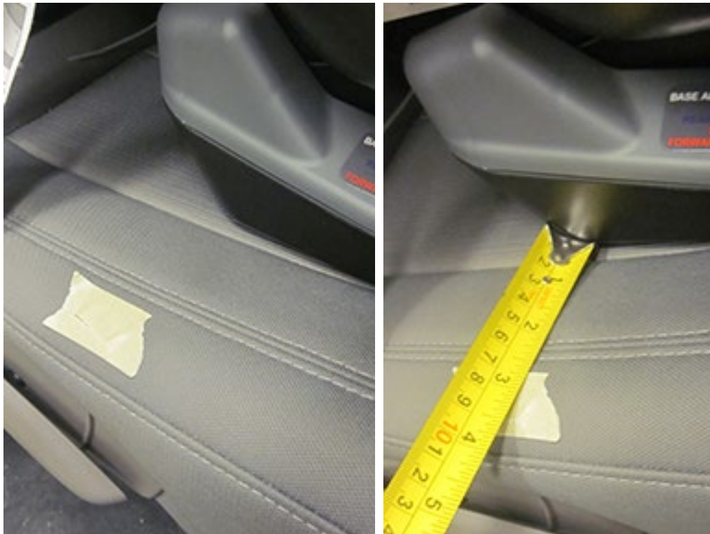
Figure 22. Measuring the amount of movement at the belt path
