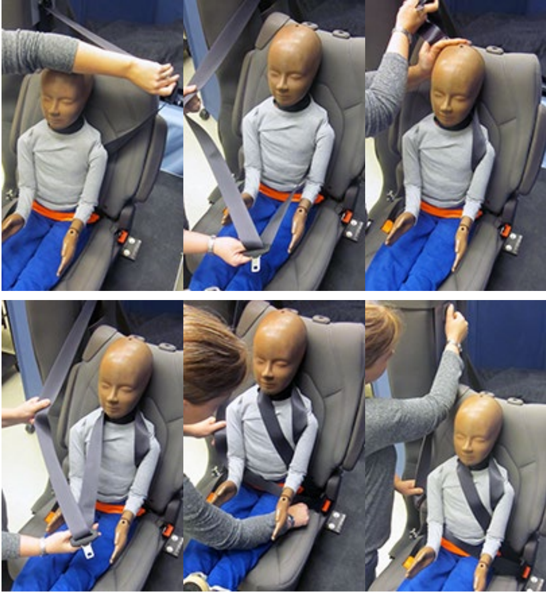
Figure 14. Steps to entangle a child surrogate routing the lower portion of the belt behind the ATD, under the left arm and then around the back of the neck (top row) and then crossing the upper portion of the belt across the chest to the buckle and engaging the ALR (bottom row)
