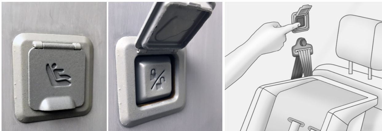
Figure 5. “Buckle-button Control” is a button that when pressed locks the retractor if the belt is buckled. The retractor is unlocked by pushing the button again or by releasing the buckle.
