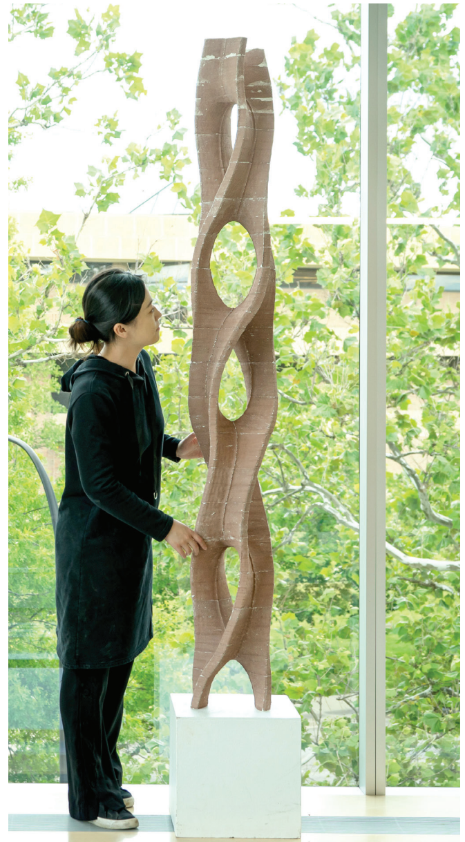
2 The resultant casts of 3D printed clay formwork, stacked, create a geometrically complex concrete column 2m in height
