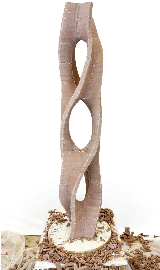
10 The final resultant cast after demolding with 1.3m height
