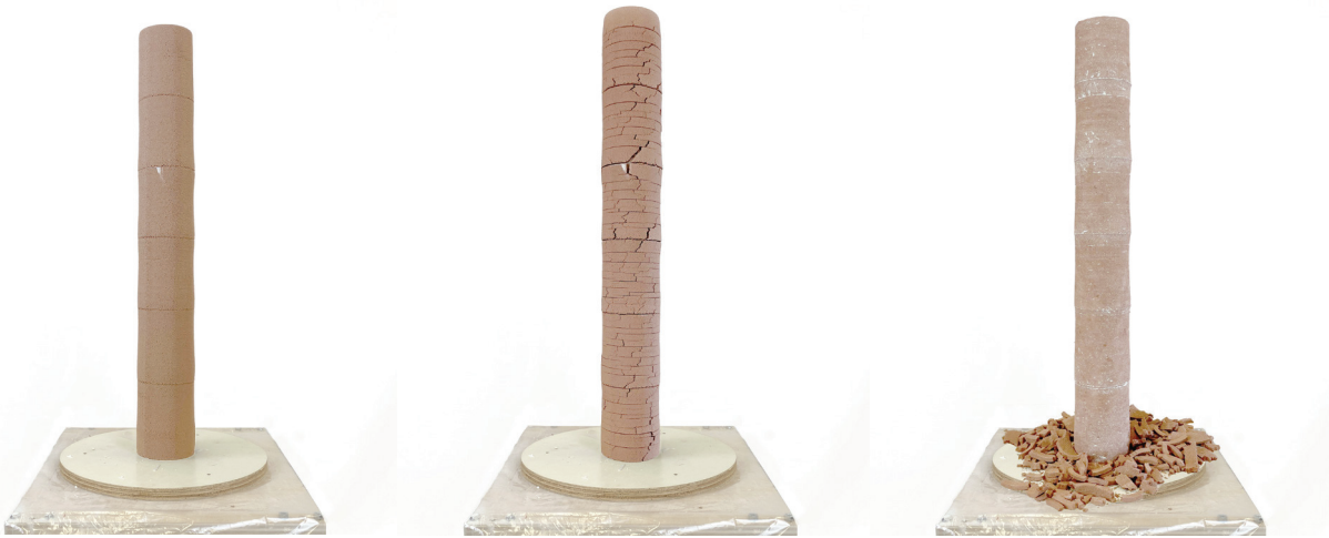
3 Sequential images showcase clay formwork, self-demolding dried clay and resultant cast.
