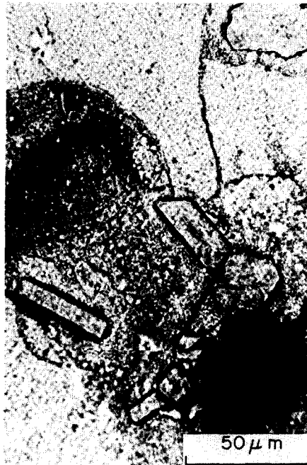
Fig. 9. Large crystals growing in a droplet on stage 7.
