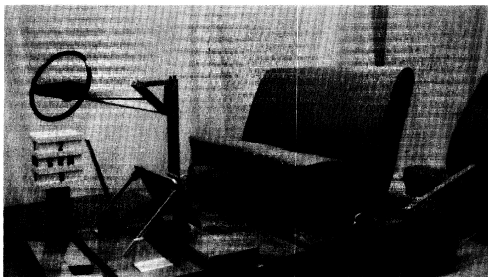
FIGURE 3-7. Phase II measurement buck with Malibu seat, toeboard, and steering wheel swung out of position.
