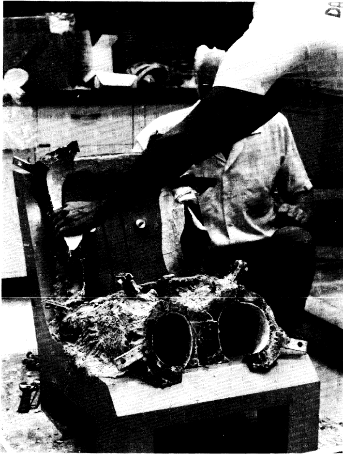
FIGURE 4-15. Assembling mold parts on hardseat to lay-up back side of shell using seat as the mold.
