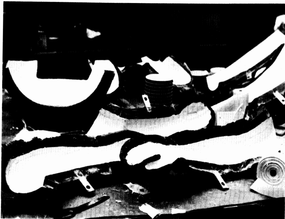
FIGURE 4-14. Laying up epoxy/fiberglass in mold parts.
