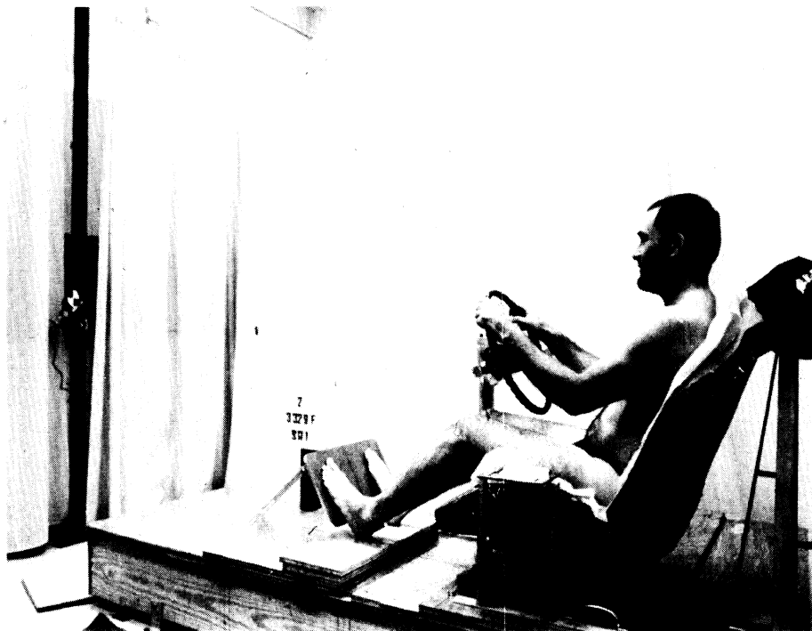
FIGURE 3-13. Mid-sized male seated in Scotchcast on vehicle seat. Scotchcast is attached to aluminum frame before it hardens.
