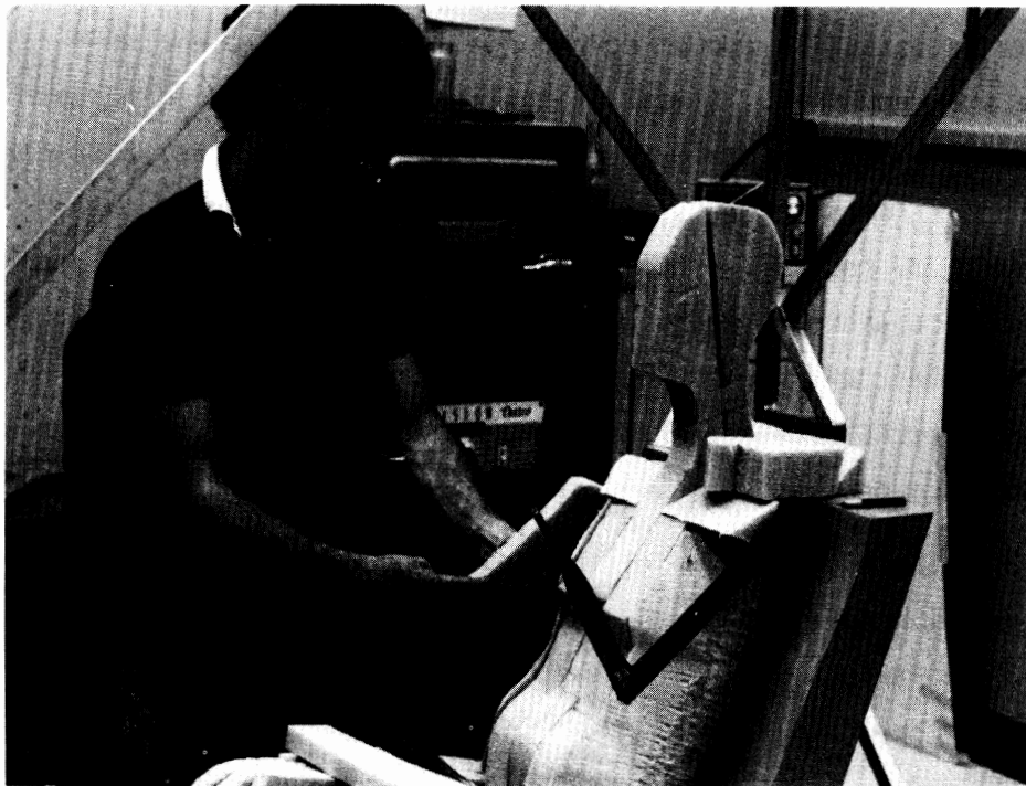
FIGURE 4-4. Attaching styrofoam to welded steel armature.
