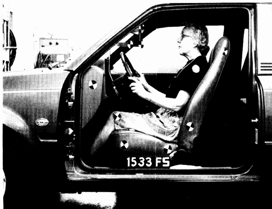
FIGURE 3-4. Small female subject sitting in Ford Escort showing a significant difference between "normal" (above) and "standardized" (below) seated postures.
