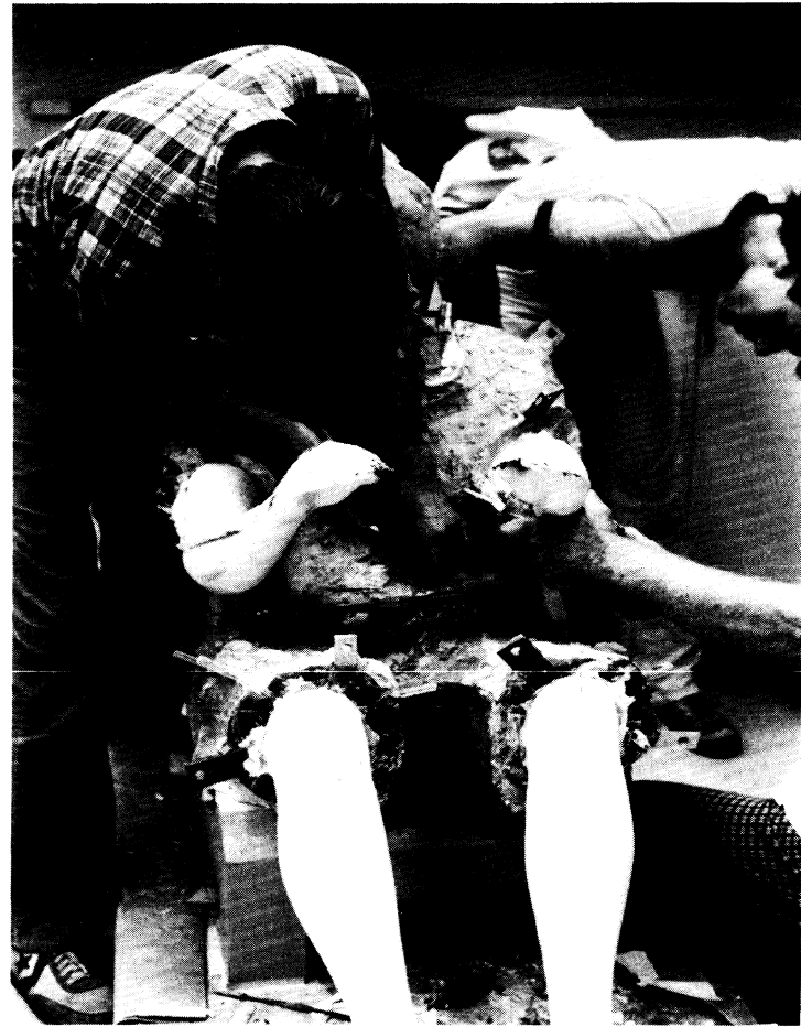
FIGURE 4-16. Removing mold parts from assembled shell.
