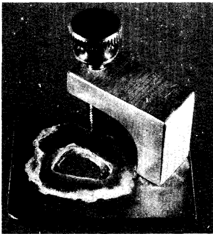
Fig. 1. The custom-adapter permitted consistent alignment of the samples to be maintained in the illuminating beam of the spectrophotometer.
