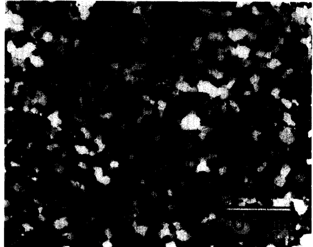
Fig. 1. Grain structure in polarized light of as-hot-pressed MoSi 2 , hot pressed at 1700 °C for 1 h under 29.4 MPa. The average grain size is 30 \mu\text{m} .
