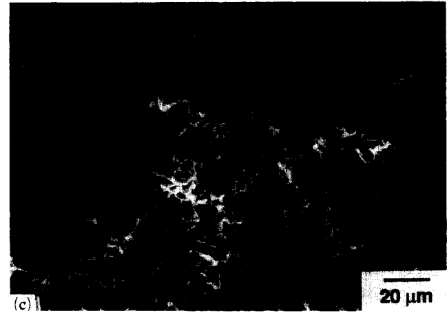
Fig. 9. SEM fractographs of 2014Al/15vol.%Al 2 O 3 under uniaxial tension test with a strain rate of 0.1 \text{ s}^{-1} at (a) 300 °C, (b) 400 °C and (c) 500 °C. The fracture mode is intergranular at 500 °C, and ductile “dimple” type at 300 °C and 400 °C.
