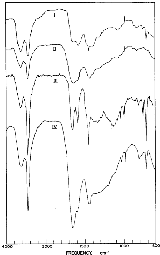
FIG. 1. Infra-red absorption spectra of the films made from treated products of the electrolysis (I, II) or LiAlH 4 reduction (III, IV) of solutions of AlCl 3 in pyridine I: dried at 50–60°C.; II: dried at 200°C.; III: dried at 60°C.; IV: dried at 200°C.
