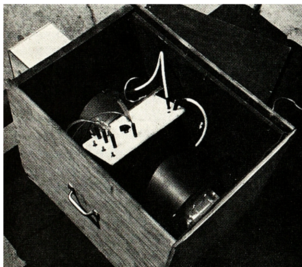
Fig. 3. Photograph of the image tube and scintillator assembly in place within its light-tight box (cover removed).
