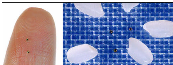
Figure 4.15 RFID chip The smallest RFID chip is 0.4mm square. Compared to a finger (left) and rice (right).
