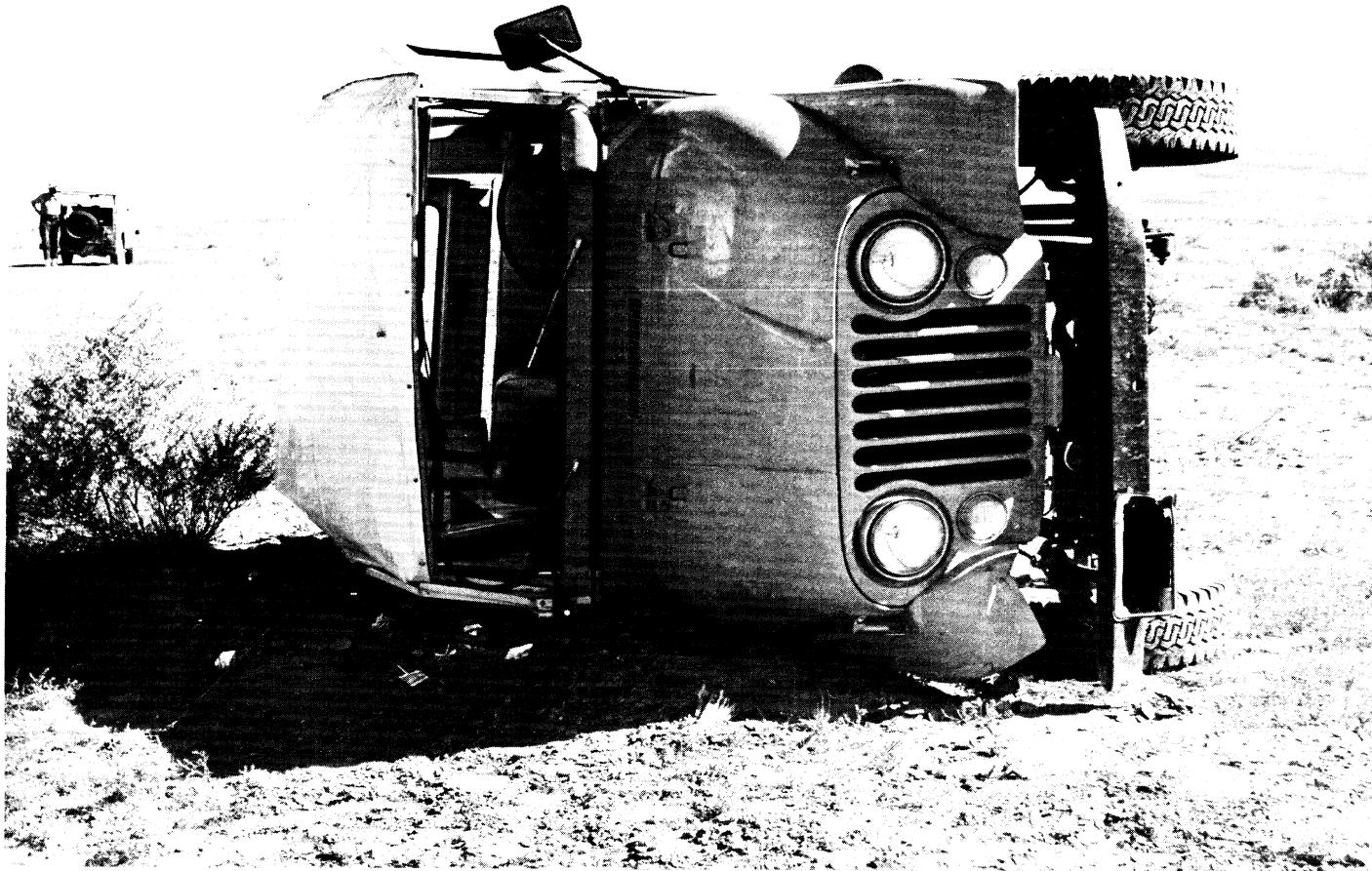
Figure 4.4.2-19 The driver of this 1974 AMC CJ-5 JEEP lost control on a curve and the vehicle rolled 1-1/2 times down an embankment, partially ejecting and fatally rolling on the right front passenger. The roll-bar effectively prevented crushing of the top; however, no shoulder harnesses were installed, and none of the three occupants were wearing the lap belt provided.
