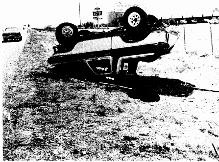
Figure 4.4.2-1 The driver of this 1978 Ford Bronco lost control at an estimated 55-60 mph entering a freeway and rolled several times. The unrestrained 25-year-old male driver was ejected through the driver's door window. Occupant restraints were installed but not used in this vehicle.
