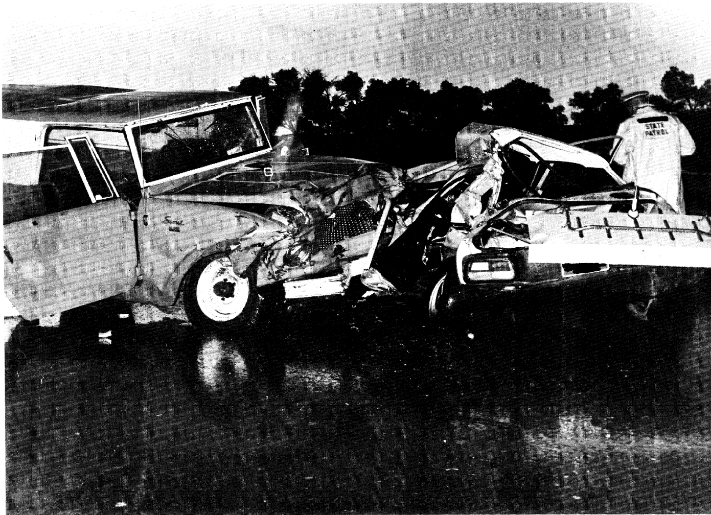
Figure 4.4.2-12 This 1965 International Scout collided with a 1975 Triumph TR-7 which had hydroplaned and skidded out of control at high speed, resulting in fatal injury to the TR-7 occupants. The Scout had no roll-bar. A lap belt restraint was used by the injured driver.
