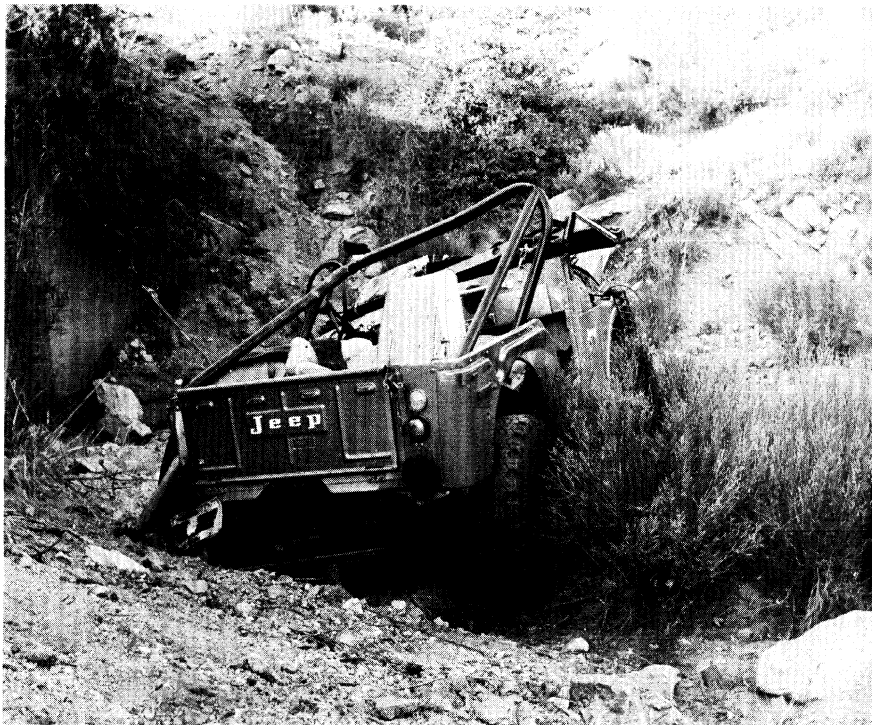
Figure 4.4.2-4 The driver of this 1974 CJ-5 JEEP lost control on loose gravel, and overcorrected. The vehicle skidded broadside toward opposite shoulder, went airborne for 16 feet, rolled over, hit a culvert, and dropped vertically 20 feet. The seat belt was fastened and the driver was not ejected, but no upper torso belt was installed. Death was due to a fractured neck and head injuries as the driver flailed during rollover.
