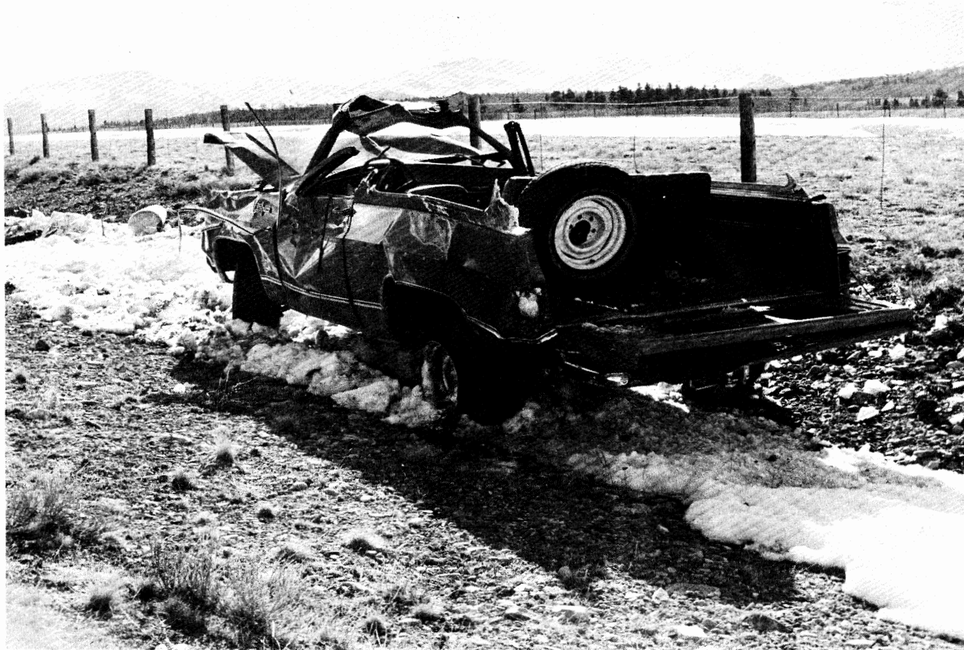
Figure 4.4.2-18 Three unrestrained occupants were ejected, one fatally, from this 1973 Chevrolet Blazer when the driver lost control and the vehicle rolled over twice. It was not equipped with a roll-bar or shoulder harness. The lap belts were not used.
