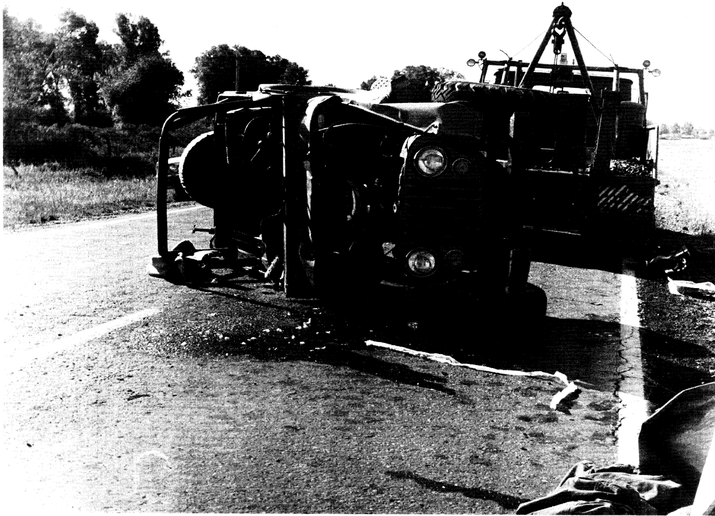
Figure 4.4.2-20 The driver was killed and the passenger injured when both, unrestrained, were ejected from this 1972 AMC CJ-4 JEEP as it rolled over two times. The original equipment roll-bar remained intact.
