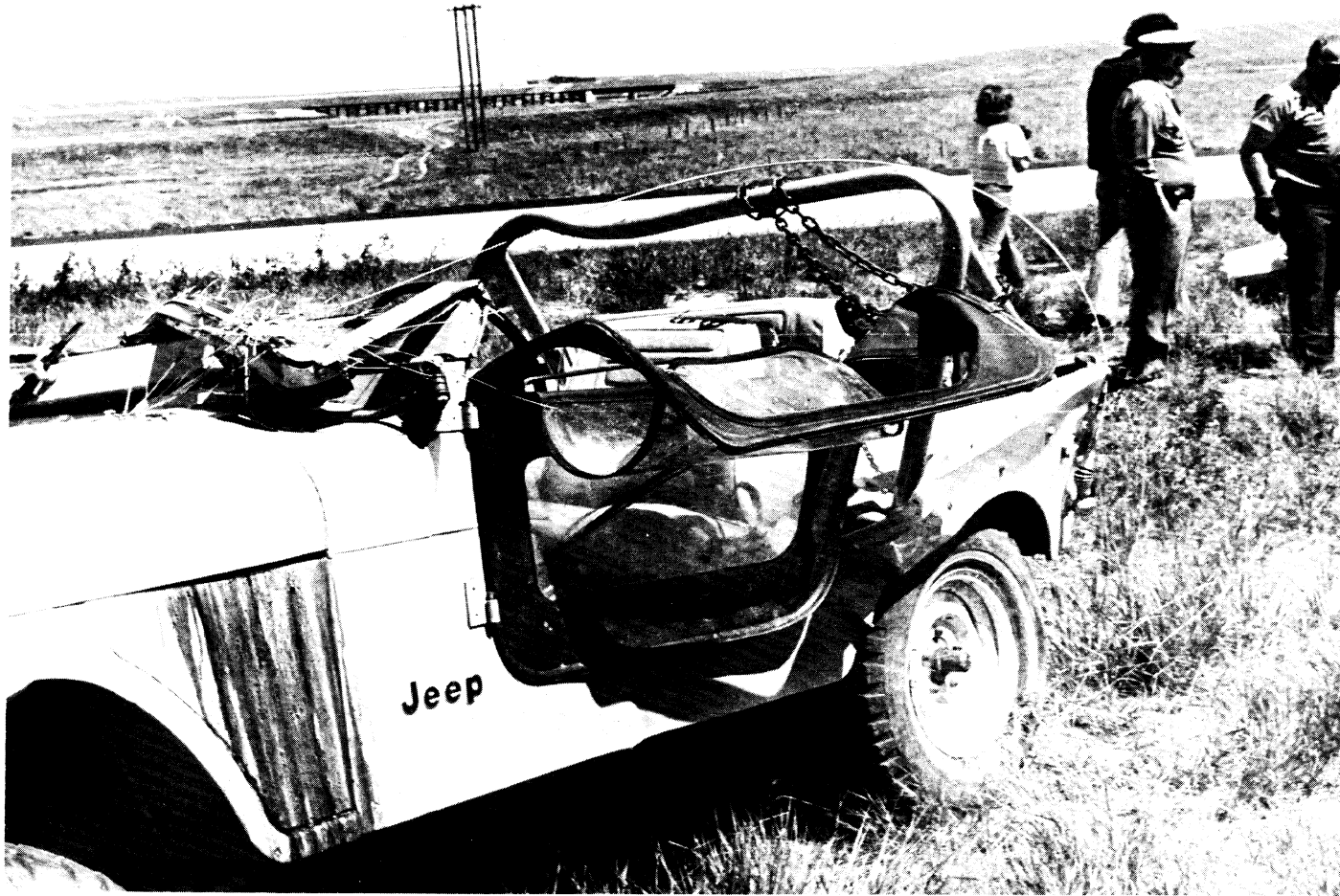
Figure 4.4.2-21 This 1976 AMC CJ-7 JEEP was struck from the rear and rolled over. Serious injury to the unrestrained passenger occurred in ejection, and the driver received fatal injuries. Although deformed, original equipment roll-bar remained intact. There were no shoulder harnesses and the occupants were not wearing lap belts.
