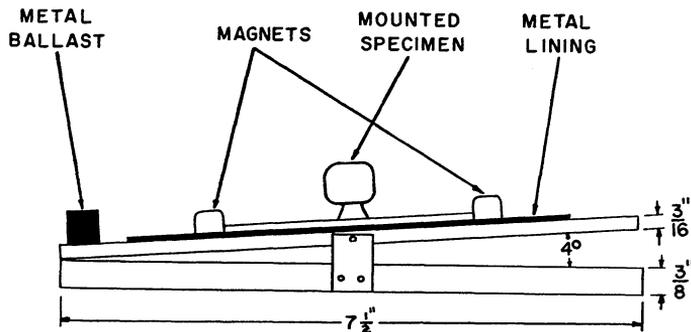
FIG. 1. Diagram of device used for single-lens stereophotography.
