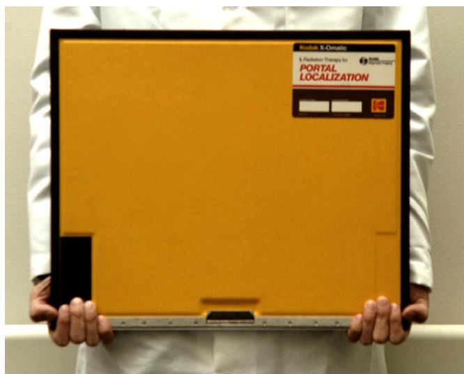
Figure 1. Picture of a radiotherapy film cassette. Such devices typically have dimensions of approximately 35 cm × 43 cm × 1.4 cm.
