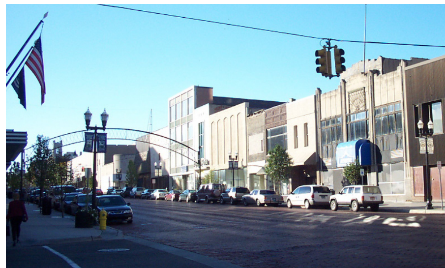
Figure 6.9: Saginaw Street, in downtown Flint, includes a number of streetscape elements, such as lampposts, street trees, and trash cans, that help separate pedestrian space from vehicle space and contribute to a pleasant atmosphere.
