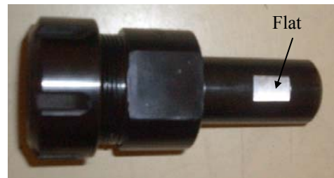
Figure 33. The collet holder with a flat machined into the shank.
