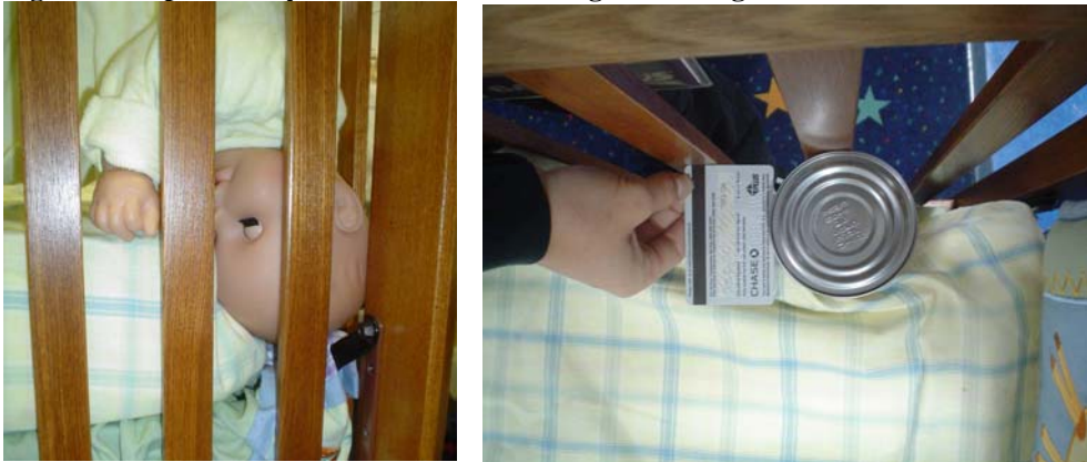
Figure 1: Gaps Already Present within Existing Crib Design Prior to Hardware Failure
