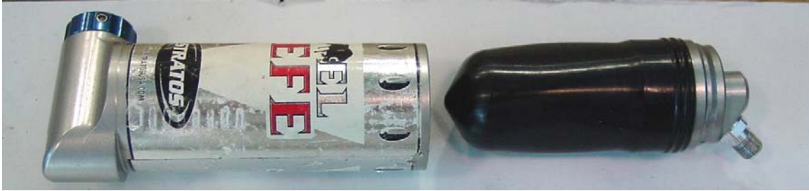
Figure 42: Example of a "bladder" to contain the pressurized gas charge.
