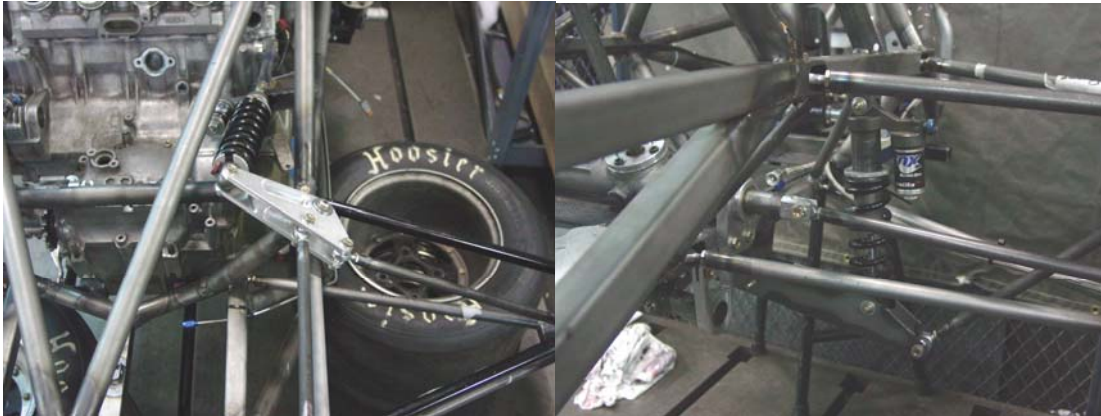
Figure 6: Location of right-side dampers in FSAE car (rear in left picture, front on right)
