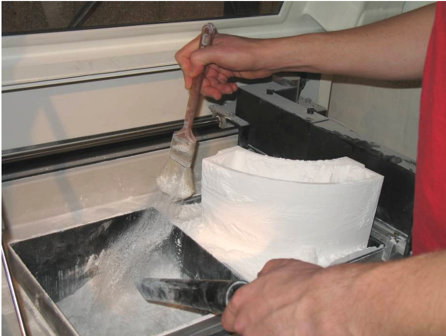
Figure F1. Finished Part Being Removed from 3D Printing Machine
