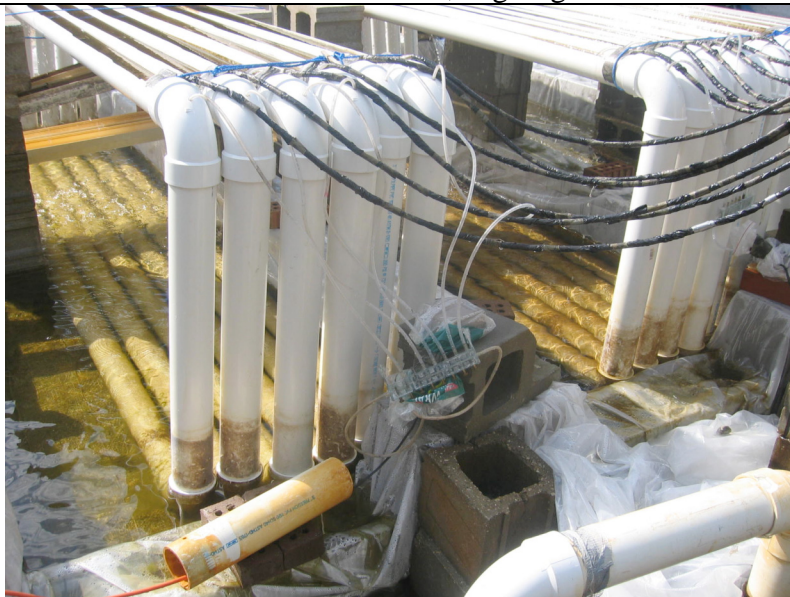
Air pump set-up to get the water to recirculate in the flumes
