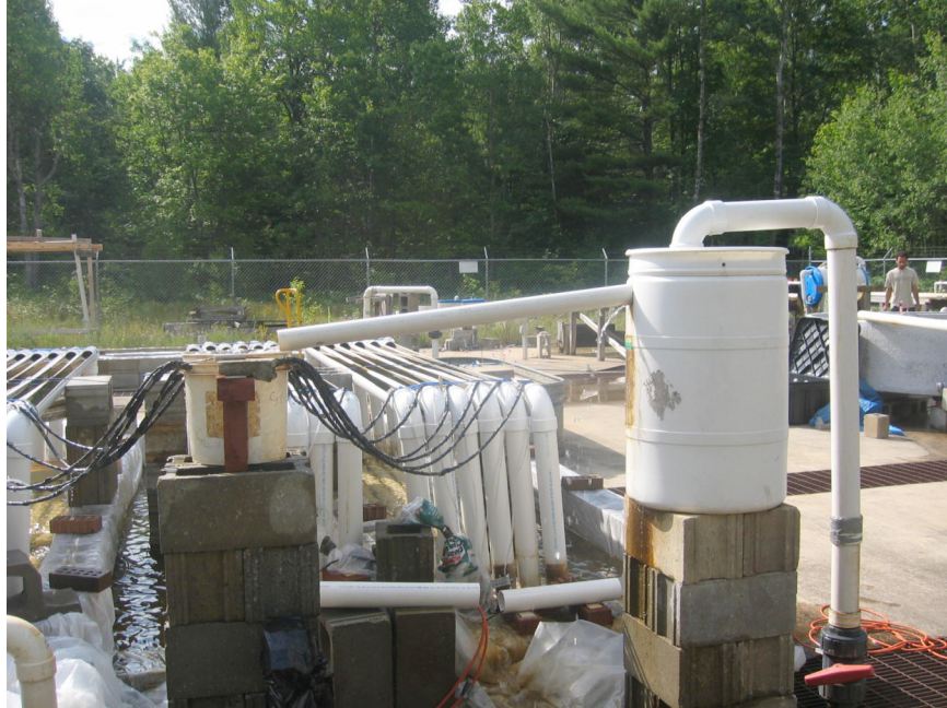
Water flowing into the bucket and then to the flumes through vinyl tubing
