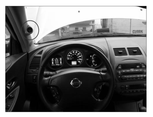
Figure 2. Inside an RDCW FOT vehicle. One camera was retrofitted to the A-pillar (circled in the figure).
