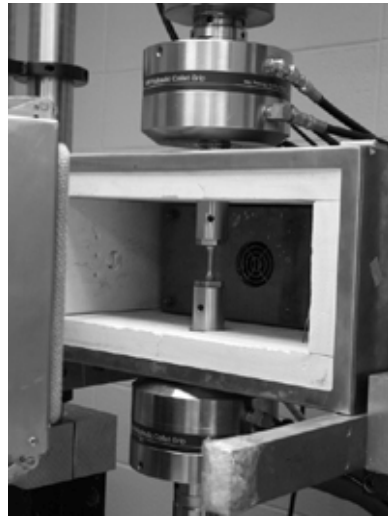
Figure 3.11 Conventional fatigue testing system equipped with an electric furnace.
