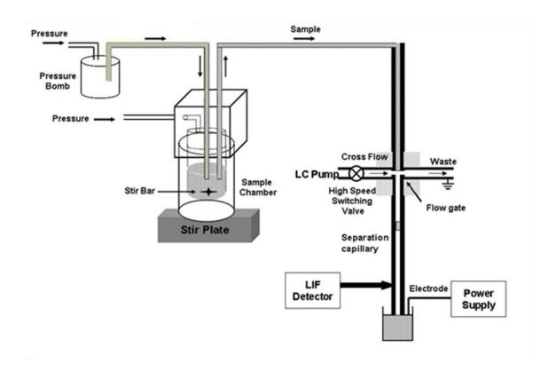
Figure 2-1. Schematic drawing of the high speed CE instrument used for kinetics studies. For the CE assays, the sample mixing system was not used. Figure adapted from source.<sup>87</sup>
