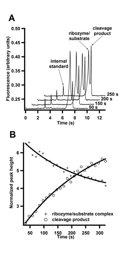
Figure 2-5. 500  $\mu$ M GlcN6P detection by CE measured in 50 mM HEPES-KOH, pH 7.5, 200 mM KCl, 25 mM DTT, 20 mM MgCl<sub>2</sub>, 500 nM singly labeled substrate, 1  $\mu$ M glmS ribozyme, 25 °C. A. Electropherograms of ribozyme cleavage. B. Fit of ribozyme cleavage rate as measured by CE, which is in good agreement with rate determined by FRET.  $k=0.0052\pm0.0002~s^{-1}$ .
