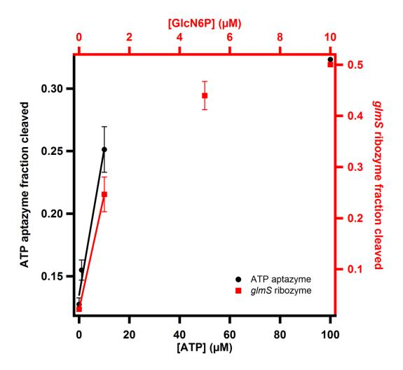
Figure 4-3. Calibration curve for multiplexed assay of ATP (●) and GlcN6P (■).
