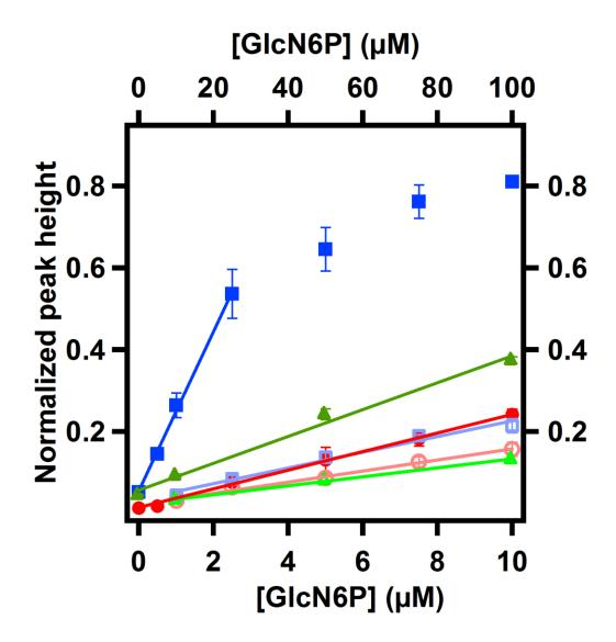
Figure 2-6. CE calibration. Left and bottom axes and closed symbols represent low concentration GlcN6P samples. Right and top axes and open symbols represent high concentration GlcN6P samples. Single-turnover samples are represented by blue squares, multiple-turnover (50  $^{\circ}$ C) by red circles, and multiple-turnover (cycled) by green triangles.
