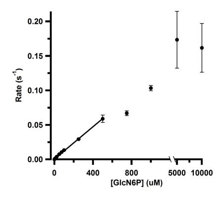
Figure 2-4. FRET calibration curve. Response is based on rate of cleavage reaction, which increases linearly up to 500  $\mu$ M with an R<sup>2</sup> value of 0.999. The limit of detection is 0.8  $\mu$ M.
