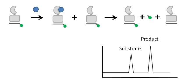
Figure 1-2: CE response to ribozyme cleavage. After cleavage reaction, uncleaved substrate is separated from fluorescent cleavage product.
