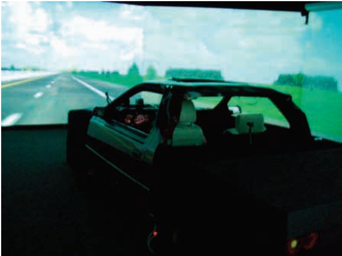
Figure 38. Simulator cab, front screen, front-right screen, and front-side screen
