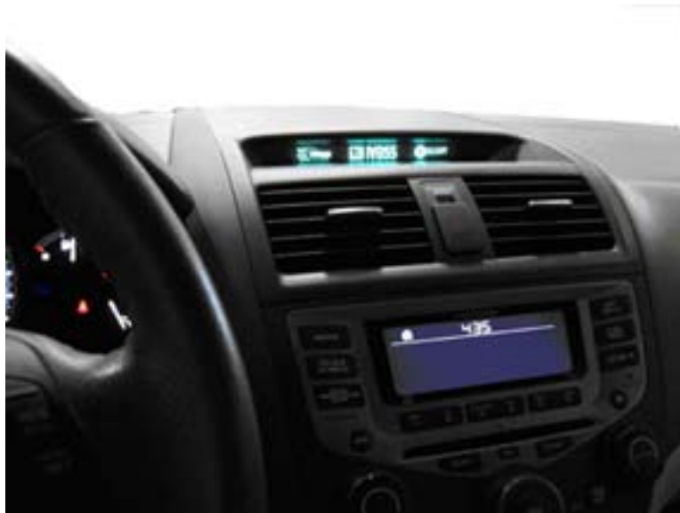
Figure 4. Center stack visual display for advisory information
