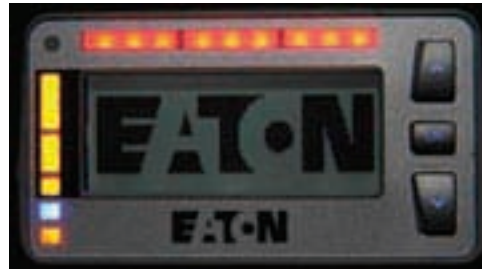
Figure 7. VORAD driver interface unit
