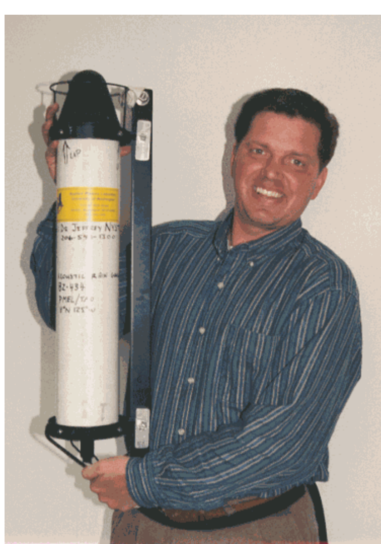
Figure 3. Dr. Jeffrey A. Nystuen holding an Acoustic Rain Gauge (ARG). This instrument is designed to be clamped onto an oceanic mooring and will record the underwater sound for one year.
