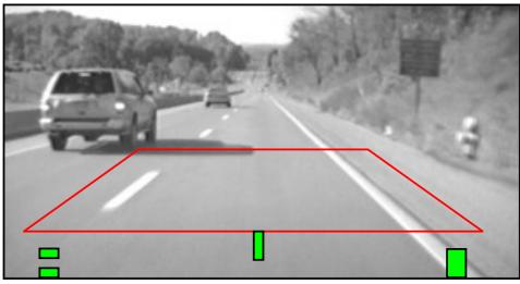
Figure 1. Camera view used to determine own vehicle's position in the road ahead (from AssistWare website).
