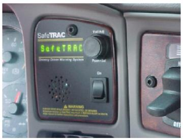
Figure 2. Factory Installation of SafeTRAC<sup>©</sup> (from AssistWare website).
