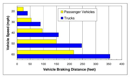
Figure 5. Comparison of passenger and HT regulated braking distances.
