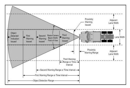
Figure 6. FMCSA recommended FCW three-stage warning thresholds and warning threshold placement zones (from Houser et al., 2005).
