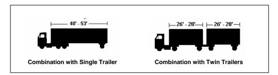
Figure 3. Typical tractor-semitrailer configurations (adapted from Harkey, Council, & Zeeger, 1996)
