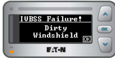
Figure 17. Display indicating windshield is too dirty for LDW subsystem to reliably determine lane position.
