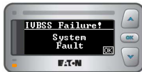
Figure 21. Display for general system fault message.
