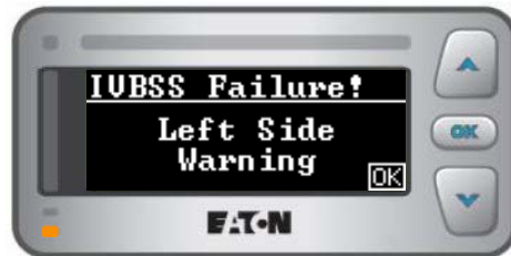
Figure 18. Display for left-side channel fault detected in the LCM subsystem.
