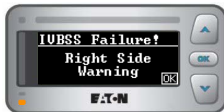
Figure 19. Display for right-side channel fault detected in the LCM subsystem.
