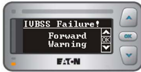
Figure 22. Example of a scroll bar, which allows the driver to view multiple system failure screens.
