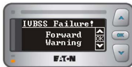
Figure 9. Display for multiple subsystem faults with scroll arrows.
