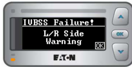
Figure 20. Display for channel fault detected in both sides of the LCM subsystem.
