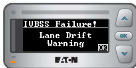
Figure 16. Display indicating a fault in the LDW subsystem.
