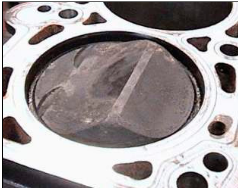
Figure 2.2: The piston is crowned with valve reliefs cut for each intake valve. This piston is shown at top dead center (TDC) location.
