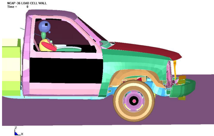
Figure 2.15 Truck with an innovative inflatable body before deployment
