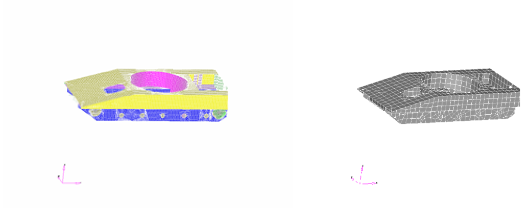
Figure 2.2 Conventional FEA and EFEA model for an Army vehicle
