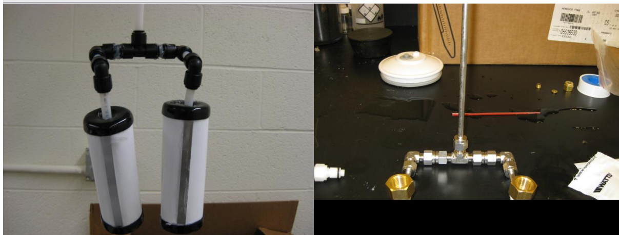
Figure 19. Internal membrane system mock up and prototypes (membrane and vacuum system on right, sparging on left).
