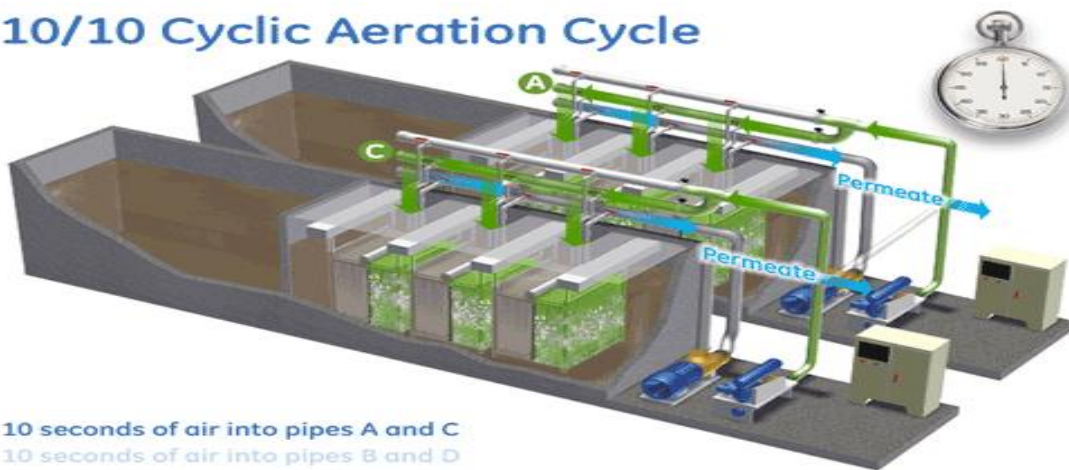
Figure 3. Employing PLC for cyclic aeration cycle [5].
