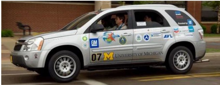
Figure 4: Hydraulic hybrid modified GM Chevy Equinox
