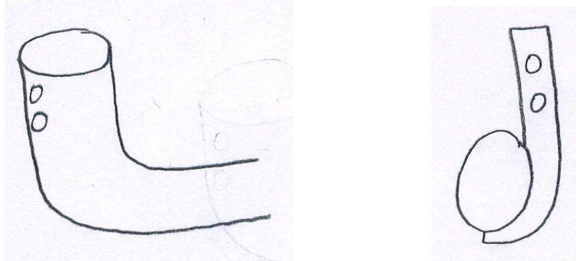
Figure C.2: Bend the trailer hitch bar up (left) and snorkel bracket (right)
