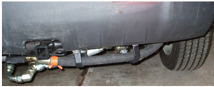
Figure 1: Final trailer hitch design integrated into the hydraulic hybrid vehicle
