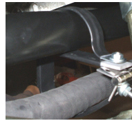
Figure 2: Attachment supporting hydraulic line in vehicle
