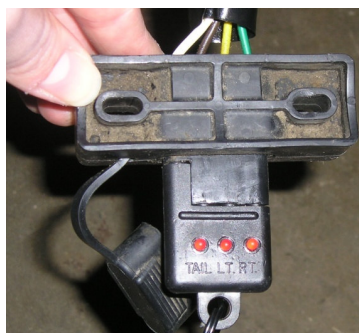
Figure 40: 4-Wire Flat Tester
