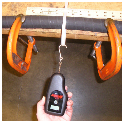
Figure 39: Pull test setup to measure deflection of hydraulic line
