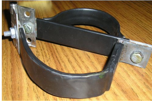
Figure 41: Corrosion tested hydraulic line attachment
