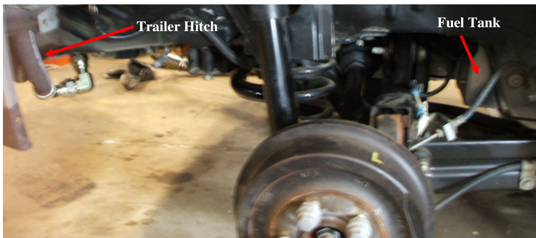
Figure 11: Fuel tank location relative to trailer hitch
