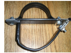
Figure 3: Manufactured hydraulic line attachment
