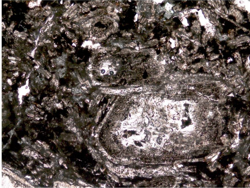
Figure 2-15: Photomicrograph of basalt dyke intruded along fault plane at Whip-5. Plane-polarized light. Note relict zoned plagioclase phenocryst in undeformed matrix of altered plagioclase laths and extensive Fe-oxide alteration. Field of view is 3 mm wide.
