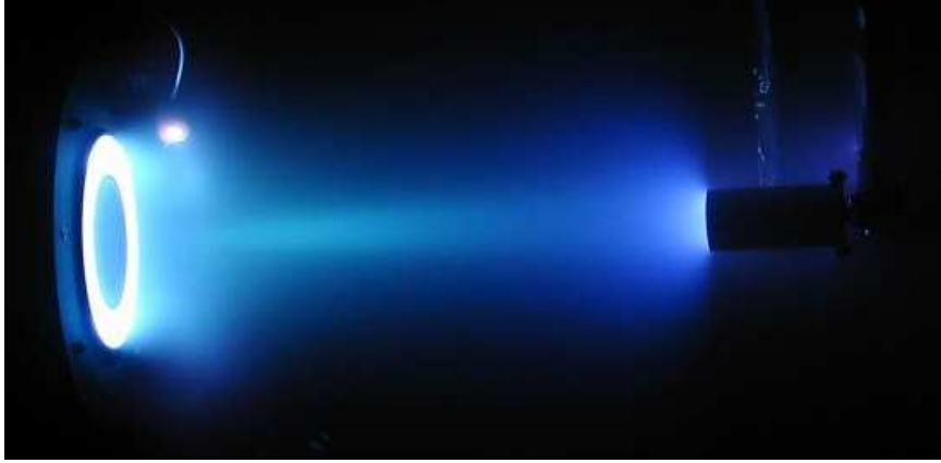
Figure 1.2: Photograph of a Hall thruster plume interacting with a Faraday probe [11].
