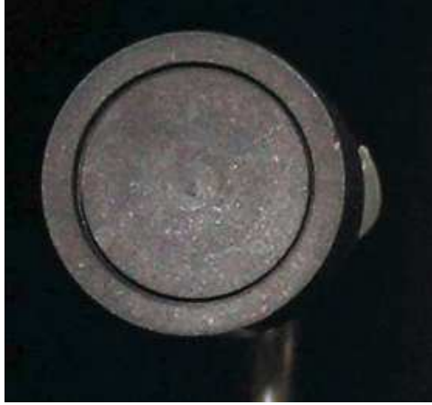
Figure 5.1: Faraday probe used in experimental BHT-200 measurements [77].
