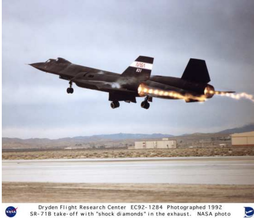
Figure 5.7: Shock diamonds in the exhaust of the SR-71 Blackbird. Credit: NASA.
