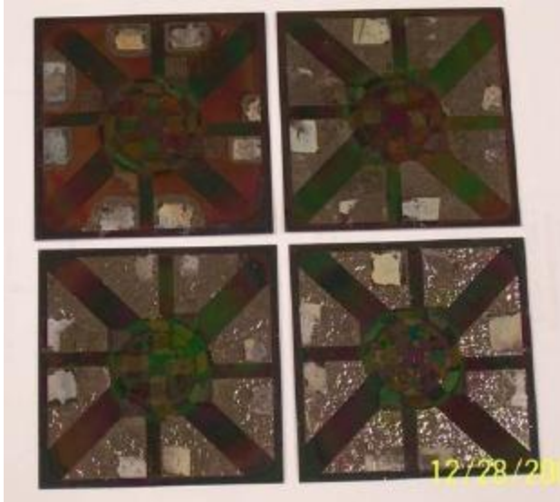
Figure 6-14: Sample set EM01 showing stress-induced buckling of encapsulation schemes after 48 hours in 85°C/85% testing chamber
