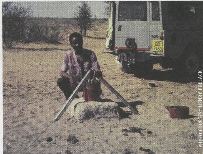
An assistant to Geology Professor Henry Pollack uses a borehole in Niger to measure the earth’s past temperatures.
