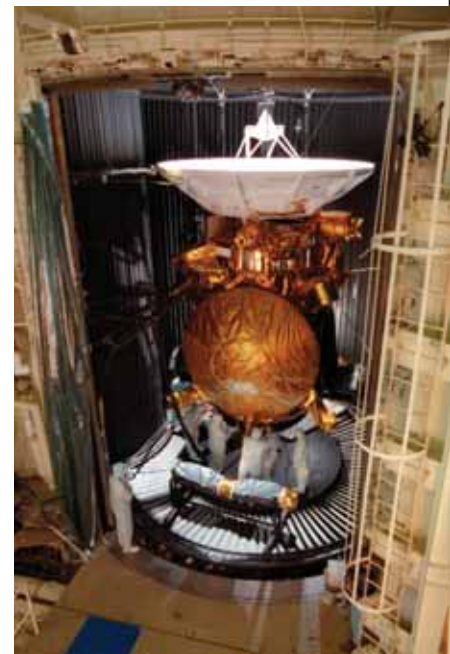
THE HUYGENS PROBE IS INSTALLED IN THE CASSINI ORBITER AT THE KENNEDY SPACE CENTER. COURTESY OF NASA.
